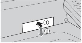
Insert a PCMCIA/PC card into the PCMCIA/ PC Card slot as illustrated. (Label side up)
